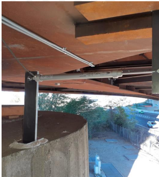
SINGLE-DIRECTIONAL DISPLACEMENT TRANSDUCERS (SR= 1 Hz)
