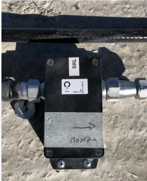
TRI-AXIAL ACCELEROMETERS (sampling rate = 125 Hz)
