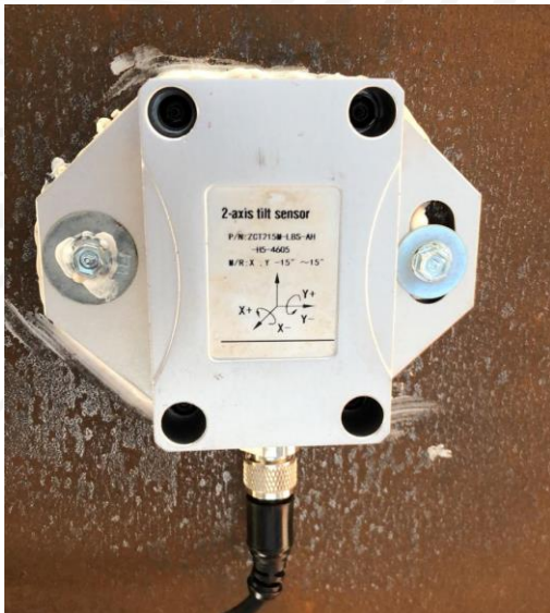
BI-AXIAL INCLINOMETERS (sampling rate = 1 Hz)
